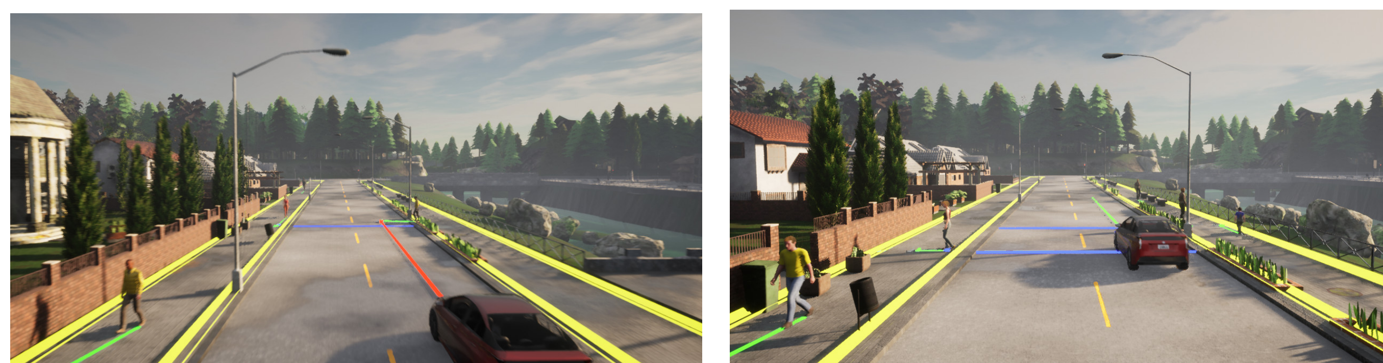
Figure 3. Pedestrian Prediction Scenario. We use the CARLA driving simulator [4]. Pedestrians spawn on the sidewalk (yellow region) and the ego (red) car predicts the pedestrian trajectories within the next 3 seconds (green). Some pedestrians will cross the road at right angles. Left: the planner predicts a collision with a crossing pedestrian and starts slowing (red ego drives up to the blue crossing line but not further). Right: ego is safely passing the road segment where the pedestrian has already crossed.
